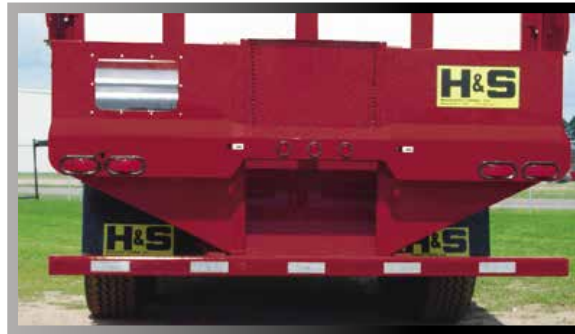
An optional grain hopper gravity unload for small grains is available for wide body boxes with a top hinged gate.
