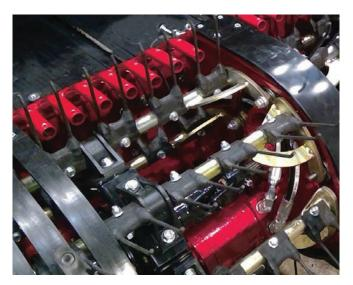
**RUBBER-MOUNTED TEETH**Hay Strippers removed for viewing
