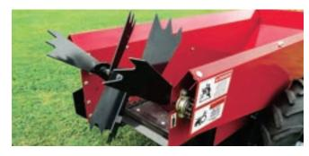
The 20" diameter, 8-paddle beater on the **\$1225** provides an even spread of material.
