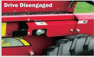
To engage the beater and main apron on the **\$1250** and **\$1280**, lower the control lever.
