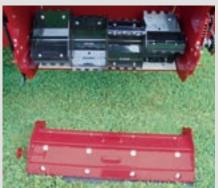
The heavy-duty expeller system, with a quick release polylined fine spread pan and side fins, helps cut the drift of material towards the tractor and spreader and provides an excellent spread pattern.
