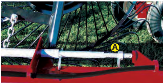
ADJUST FOR CONDITIONS Adjustment for the ground pressure on the rake wheels (A) allows the operator to fine-tune the HC5114 wheel rake to fit varying conditions.
