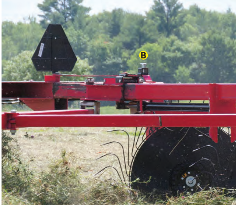
HYDRAULICALLY ADJUSTED RAKING WIDTH Setting the spring loaded stop allows you to set a pre-determined raking width (B) up to 28' on the HC5114 and 32' on the 16-wheel. Raking widths can be hydraulically adjusted in any position up to the pre-determined raking width.
