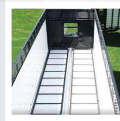
All **Wide Body** boxes have <sup>1</sup>/2" thick virgin grade solid poly with rectangular tubular steel on the outside and C-channels in the center that run lengthwise under the floor for added strength.
