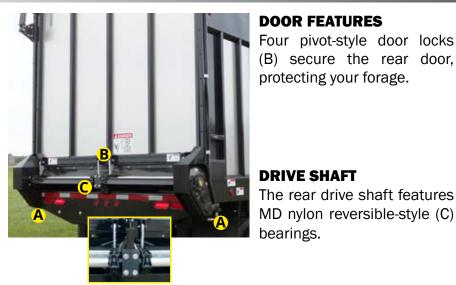
**REAR DRIVE FEATURES** All BIG DOG & TOP DOG models feature large 1" steel hydraulic lines to the rear dual hydraulic motors (A).
