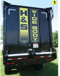
New **dual cylinder hydraulic gate delay system** allows for a fully open rear door.
