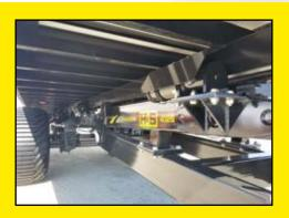
**DIGI-STAR<sup>™</sup> SCALE SYSTEM** The Digi-Star<sup>™</sup> Frame Mount Scale System (shown in above picture) is optional on all 3100 & 4100 series models.
