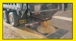
An optional quick-remove gravity unload grain hopper is available on **BIG DOG & TOP DOG** forage boxes that have a top pivot door.
