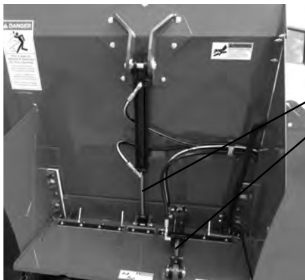
The discharge gate control cylinder shaft, discharge door deflector shield cylinder shaft and both front and rear main auger cylinders should also be frequently coated with a rust preventative spray or lubricant since the cylinder shaft may remain extended when not being used for a period of time.
