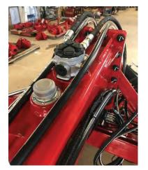
Hot Level Check Plug Hydraulic Oil Fill
