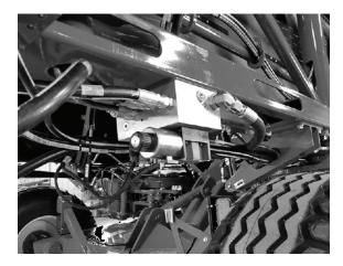
Your merger comes standard with 1 hydraulic motor to power each belt. The dual drive cross conveyor kit add and second hydraulic motor to each head. We suggest this kit units that will be merging heavy crops.
