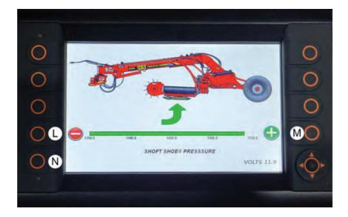
L-Used to lower the soft shoe pressure
