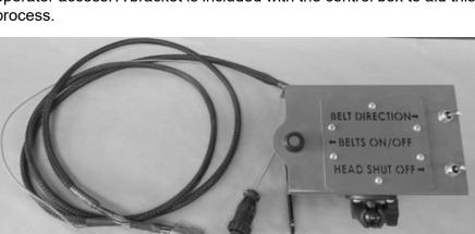
3. Connect the 3-pin cable to the tractor convenience outlet. This connection is only used for a keyed power supply for main power relay.
