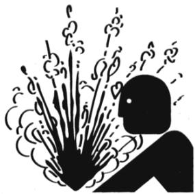
HYDRAULIC SYSTEM ON MERGER CONTAINS STORED ENERGY. RELEASING PRESSURE FROM THE ACCUMULATOR BY ANY MEANS (WELDING, TORCH, LOOSE FITTINGS) MAY RESULT IN THE RAPID RELEASE OF OIL AND/OR GAS CAUSING PERSONAL INJURY OR DEATH.
