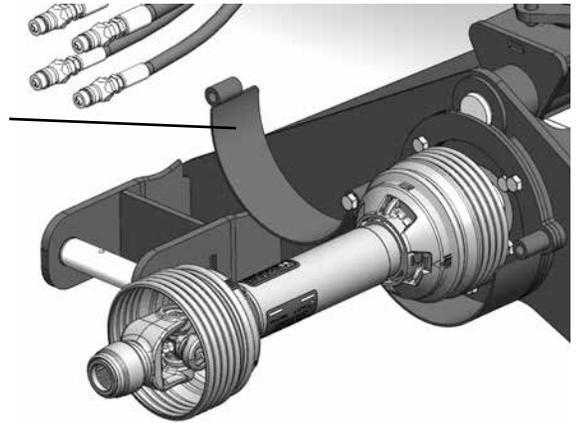
**Recommended PTO operating speed is 700-750 RPM**
