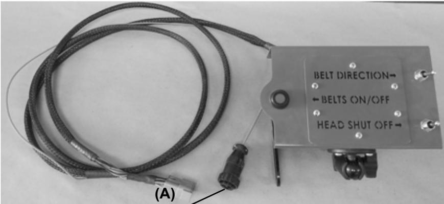
3. Connect the 3-pin cable to the tractor convenience outlet. This connection is only used for a keyed power supply for main power relay.
