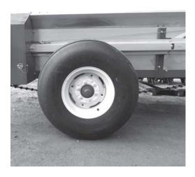
Wheel lug torque should be checked after every 50 hours of operation and tightened to the appropriate torque.
