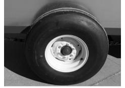
Wheel lug torque should be checked after every 50 hours of operation and tightened to the appropriate torque.
