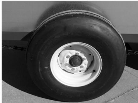
Wheel lug torque should be checked after every 50 hours of operation and tightened to the appropriate torque.
