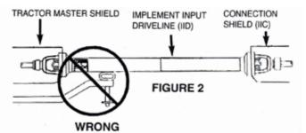
If this implement is attached to a tractor with an offset in the drawbar, be certain it is in the down position to prevent damage to the IID guarding and the IID telescoping members. [See Figure 2]
