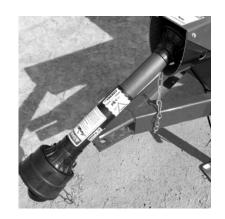
If this implement is attached to a tractor with a clevis hitch (hammer-strap) style drawbar, the hammerstrap must be removed to prevent damage to the IID guarding and the IID telescoping members. [See Figure1]
