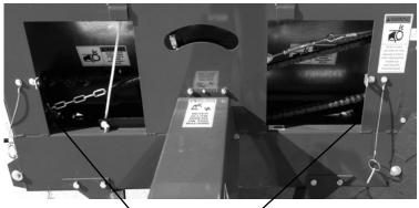
(1) on each front idler sprocket behind the shields
