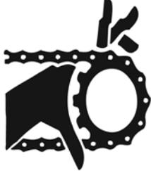
DO NOT CLEAN OR WORK ON THIS MACHINE WITHOUT FIRST DISENGAGING POWER AND SHUTTING OFF TRACTOR ENGINE.
