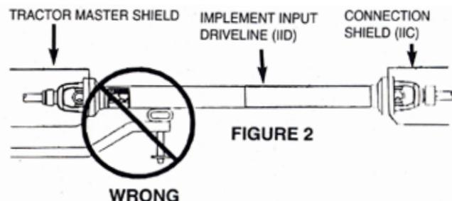
*If this implement is attached to a tractor with an offset in the drawbar, be certain it is in the down position to prevent damage to the IID guarding and the IID telescoping members. [See Figure 2]*
