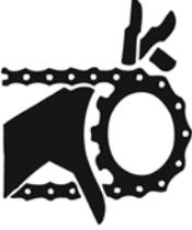
DO NOT OPERATE THIS EQUIPMENT IF THIS DECAL IS EXPOSED. REPLACE SAFETY SHIELDS.
