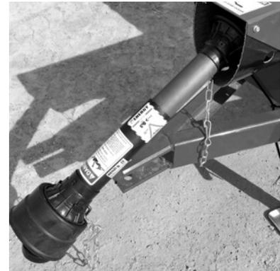
**CAUTION:** Do not use a steel hammer to aid in joining PTO parts.
