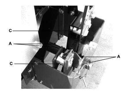
2 zerks located under shield on the pivot arm
