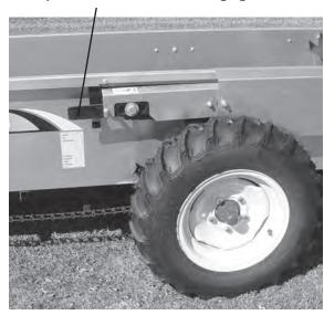
Make sure tires are mounted in correct direction as shown
