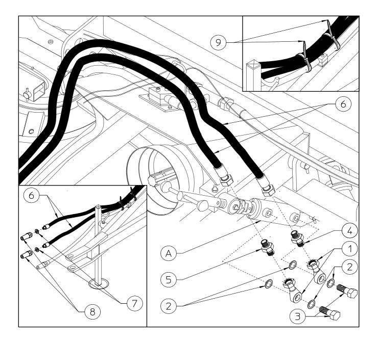
3) Connect the fittings 1 to the cylinder A using washers 2 and screws 3. Connect the reducer flow 4 to the fitting 1. Connect the nipple 5 to the fitting 1. Connect the hoses 6 to the reducer flow 4 and nipple 5. Extend hoses 6 along the drawbar until it reaches the front part. Lock the hoses 6 with clips 9. Apply the washers 7 and rapid couplings 8 to the hoses 6.
