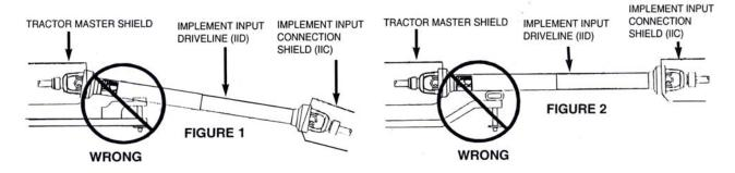
If the Tedder is attached to a tractor with an offset in the drawbar, be certain it is in the down position to prevent damage to the IID guarding and the IID telescoping members. [See Figure 2]
