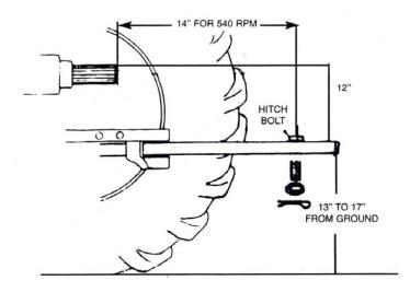
If the Tedder is attached to a tractor with a clevis hitch (hammer-strap) style drawbar, the hammer-strap must be removed to prevent damage to the IID guarding and the IID telescoping members. [See Figure 1]
