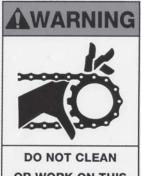
OR WORK ON THIS MACHINE WITHOUT FIRST DISENGAGING POWER AND <u>SHUTTING OFF</u> TRACTOR ENGINE.
