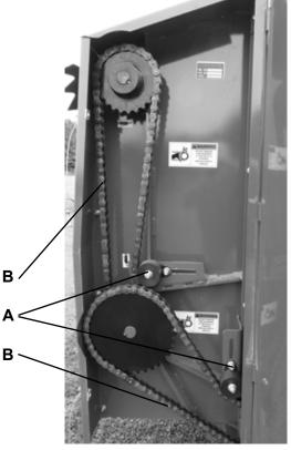
Shields Opened for Clarity NOTE: PERIODICALLY LUBRICATE ALL ROLLER CHAINS WITH A LIGHT MACHINE OIL.
