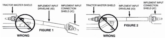
If this implement is attached to a tractor with an offset in the drawbar, be certain it is in the down position to prevent damage to the IID guarding and the IID telescoping members. [See Figure 2]
