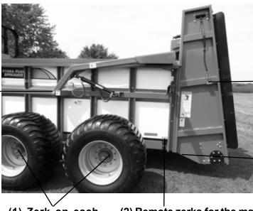
(1) Zerk on each\_ side for hydraulic end gate pivot Vertical Beater Models (2) Zerks - one for each bearing on the top of the vertical beaters
