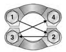
Flange Bolt Tightening Sequence
