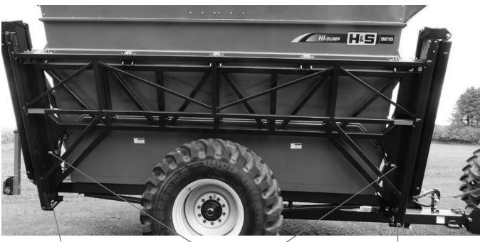
Slide Extension Roller (1) Remote Zerks / \* Box Pivots (7) Slide Extension Roller (1)
