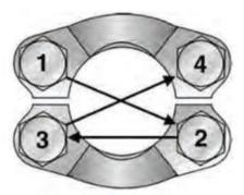
Flange Bolt Tightening Sequence
