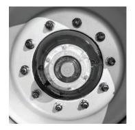
With the hub horizontal, remove the plastic cap and fill the hub cavity to the fill line with Casrtol Hyspin VG46 hydraulic oil. Replace the plastic cap.
