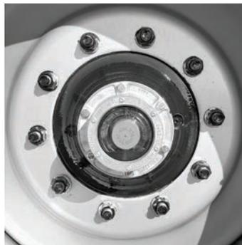
With the hub horizontal, remove the plastic cap and fill the hub cavity to the fill line with Casrtol Hyspin VG46 hydraulic oil. Replace the plastic cap.
