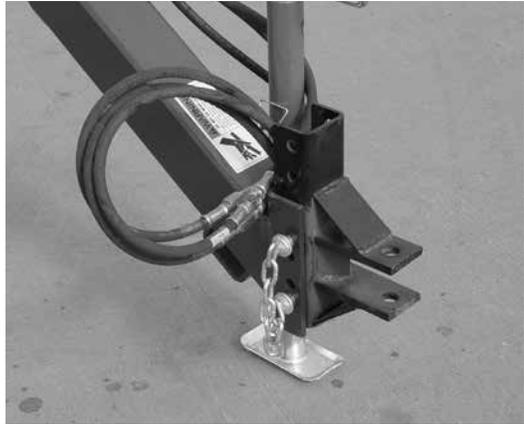
2. There are ten different positions to adjust the hitch on your new rake. Hitch should be adjusted so main frame of the rake is level or parallel to the ground.
