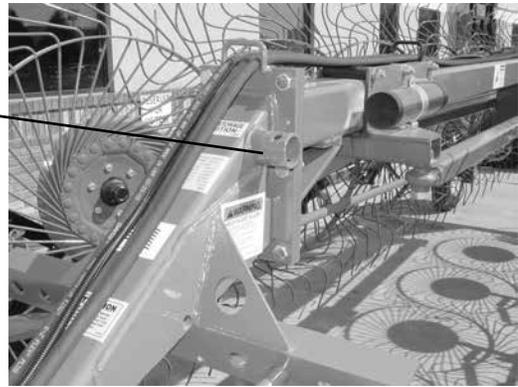
4. Connect hydraulic hose for raising and lowering rake wheels from rake to a double acting valve on the tractor.
