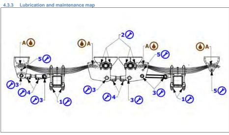
1 - Axle anchoring to leaf spring: check correct housing.
