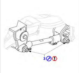
4 – End terminal screw torque check on axle reaction rods
