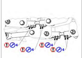
5 – Leaf spring non-slip screw torque check.
