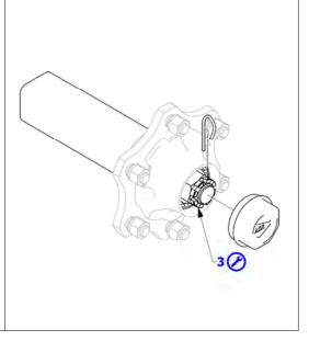
3. Bearing gap check (Teknoax version with screw-in hub cap).
