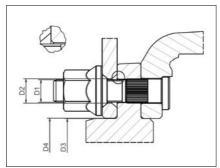
5. Single wheel with conic nut
