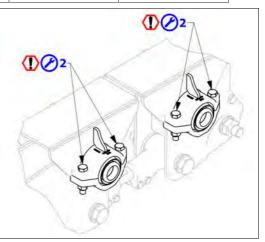
3 - Threaded pin torque check on axle reaction rods
