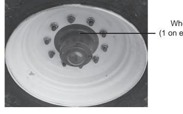
Wheel Hub Zerk (1 on each wheel hub)
