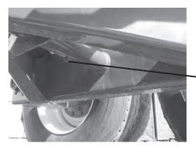
Walking Beam Pivot Zerk -(1 on each Pivot)
