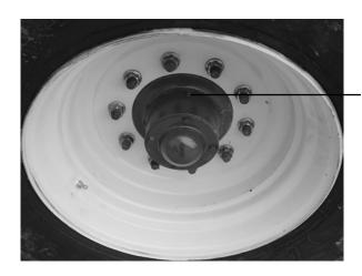
Wheel Hub Zerk (1 on each wheel hub)
