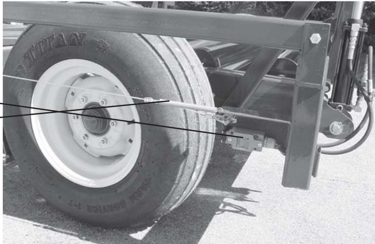
**IF THE EMERGENCY STOP IS TRIPPED DURING WRAPPING CYCLE, THE UNIT MUST BE SWITCHED TO MANUAL OPERATION ON THE CONTROL PANEL. PRESS THE START/RESET SWITCH, THEN PRESS AND HOLD THE MANUAL PUSHER AND HOOP SWITCHES TO BEGIN WRAPPING AGAIN, WHILE HOLDING SWITCHES, SELECT THE DESIRED MODE, AUTOMATIC OR REMOTE ON THE CONTROL BOX TO CONTINUE NORMAL OPERATION.**
