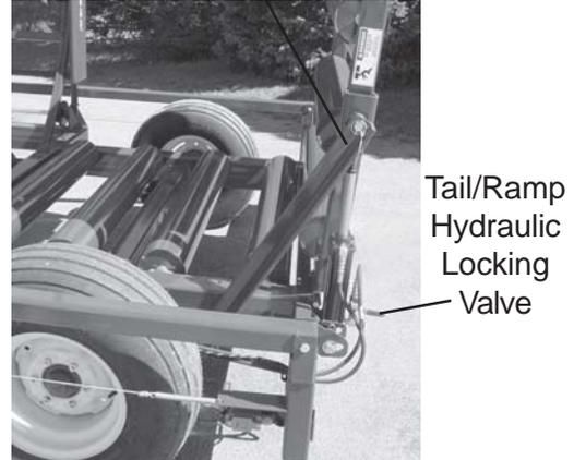
7. Activate the hydraulic control lever to lower the tail/ramp. Cycle the ramp up and down a few times to remove any air pockets. Turn the wheel brake valve to the upright or off position, lower the ramp and the wheel brake will set.
