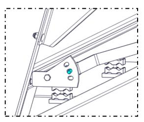
3. To produce a more even bed of straw, the pan can be twisted by forcing the end with the five holes to a lower slotted hole and the other end to the second slot which would result in varying exit speed along the length of the outlet, throwing longer on the narrowed end, throwing shorter on the more open end.
