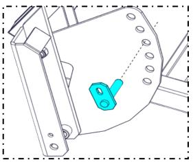
3. Install the cylinder into the cylinder mount, secure with the mounting pin (3-11/16"), 3/8" bolt, flat washer, and lock nut.
