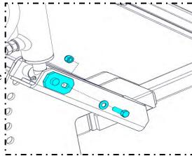
If there is excessive pressure on the deflector shield, loosen the bolts holding the top cylinder mount, and adjust its position down slightly within the slotted holes. After adjusting the top cylinder mount, recheck that the deflector does not come closer than 1" away from contacting the bale shroud. Further adjustment is available by positioning the table and support brackets as necessary.
