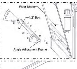
3. Now release the spring latch into the slotted holes of angle adjuster frame and fasten the bolts.
