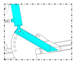
6. After making sure the deflector shield is free to move without hitting the bale shroud, retract the cylinder until it is closed. Watch to make sure that cylinder does not put excessive pressure upwards on the deflector shield in this position.
