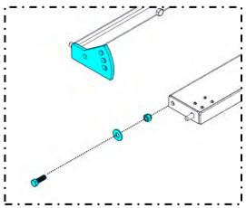
2. Install the angle adjuster frame by bolting them to the body of the Bale processor.
