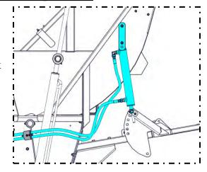
5. Extend the cylinder to its maximum point of extension, making sure that the deflector shield does not come closer than 1" away from contacting the bale shroud.
