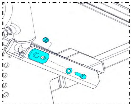
***If there is excessive pressure on the deflector shield, loosen the bolts holding the top cylinder mount, and adjust its position down slightly within the slotted holes. After adjusting the top cylinder mount, recheck that the deflector does not come closer than 1" away from contacting the bale shroud. Further adjustment is available by positioning the table and support brackets as necessary.***
