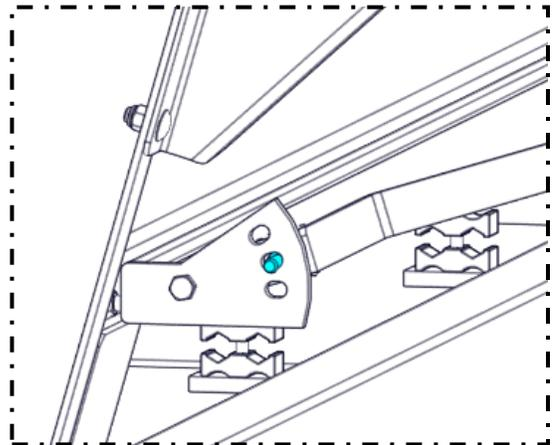
3. To produce a more even bed of straw, the pan can be twisted by forcing the end with the five holes to a lower slotted hole and the other end to the second slot which would result in varying exit speed along the length of the outlet, throwing longer on the narrowed end, throwing shorter on the more open end.
