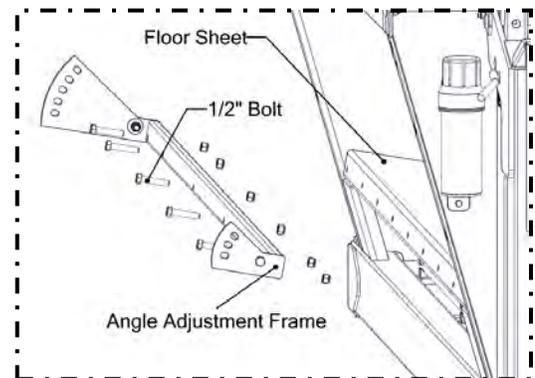
3. Now release the spring latch into the slotted holes of angle adjuster frame and fasten the bolts.
