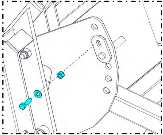
2. Use the provided 3/8" bolts, nuts, and washers to secure the mount to the shroud. Tighten the bolts with the cylinder mount pushed up as high as the slotted holes will allow.
