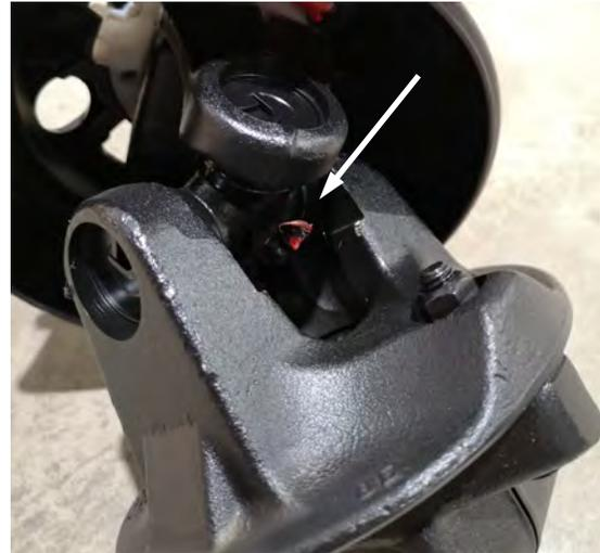
PTO, mid: grease zerk, extend PTO and rotate shield to find zerk (every 8 hours)
