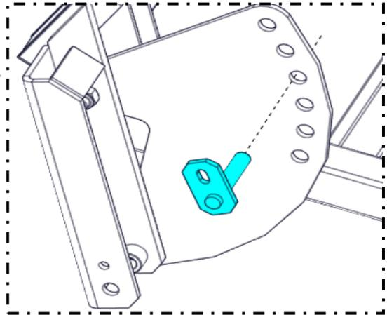
3. Install the cylinder into the cylinder mount, secure with the mounting pin (3-11/16"), 3/8" bolt, flat washer, and lock nut.
