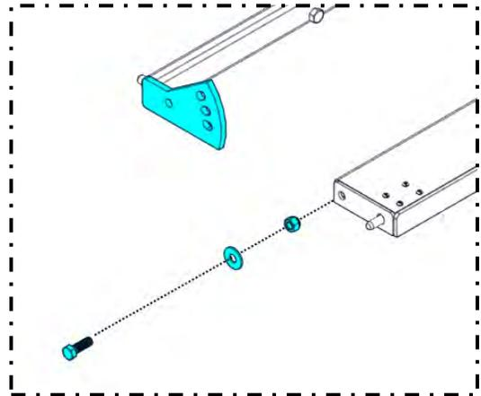
2. Install the angle adjuster frame by bolting them to the body of the Bale processor.
