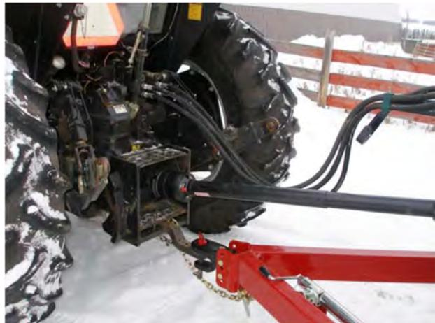
11. Route the hoses along the hitch and secure in position to prevent entanglement with any moving parts.
