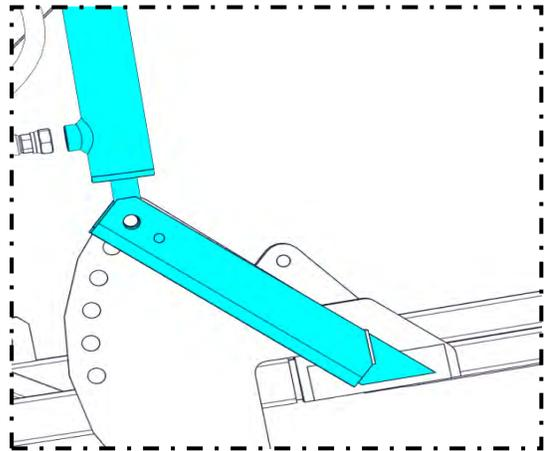
6. After making sure the deflector shield is free to move without hitting the bale shroud, retract the cylinder until it is closed. Watch to make sure that cylinder does not put excessive pressure upwards on the deflector shield in this position.
