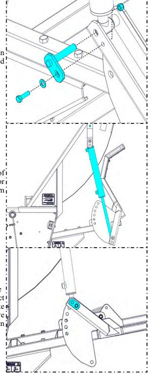
If there is excessive pressure on the deflector shield, loosen the bolts holding the top cylinder mount, and adjust its position down slightly within the slotted holes. After adjusting the top cylinder mount, recheck that the deflector does not come closer than 1" away from contacting the bale shroud. Further adjustment is available by positioning the table and support brackets as necessary.
