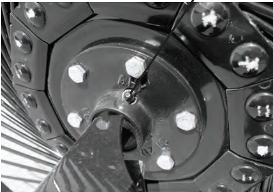
1 zerk on each rake wheel hub assembly
