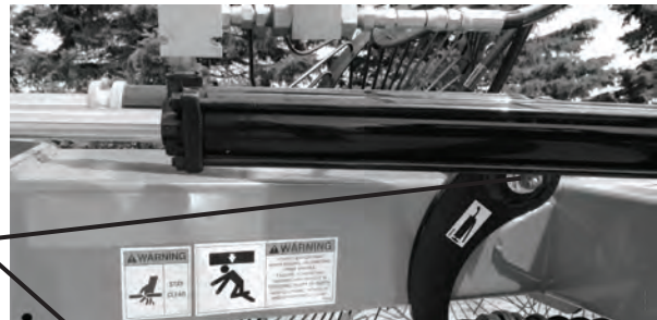
1 zerk on each of the pivot points
