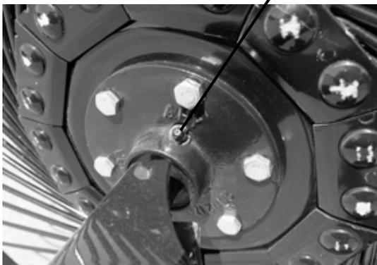
1 zerks on each of the adjuster pivot points
