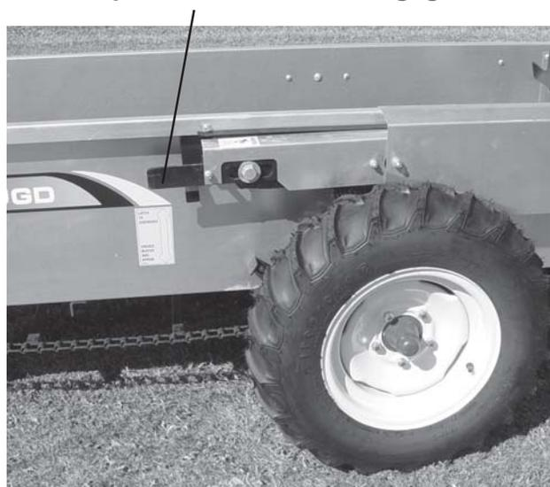
**Make sure tires are mounted in correct direction as shown**
