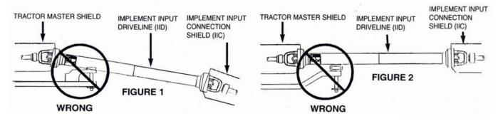
If this implement is attached to a tractor with an offset in the drawbar, be certain it is in the down position to prevent damage to the IID guarding and the IID telescoping members. [See Figure 2]
