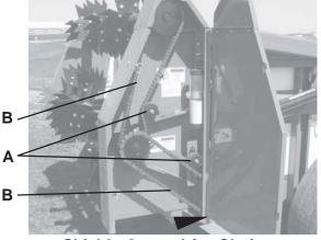
Shields Opened for Clarity NOTE: PERIODICALLY LUBRICATE ALL ROLLER CHAINS WITH A LIGHT MACHINE OIL IF NOT EQUIPPED WITH AN AUTOMATIC OILER.
