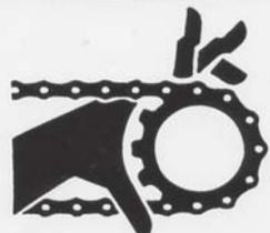
DO NOT CLEAN OR WORK ON THIS MACHINE WITHOUT FIRST DISENGAGING POWER AND **SHUTTING OFF TRACTOR ENGINE.**
