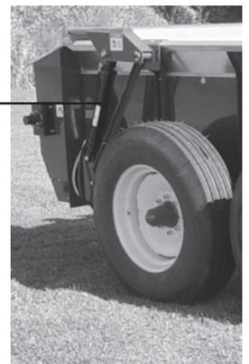
**NOTE:** DOUBLE CYLINDER FOR HYDRAULIC ENDGATE IS STANDARD EQUIPMENT FOR MODELS 3137 & 3143.
