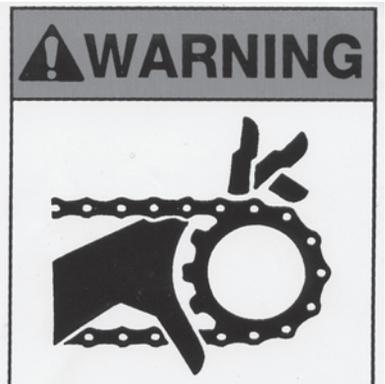
**DO NOT CLEAN OR WORK ON THIS MACHINE WITHOUT FIRST DISENGAGING POWER AND SHUTTING OFF TRACTOR ENGINE.**
