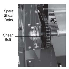
Shields Removed For Clarity
