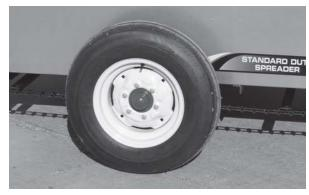
Wheel lug torque should be checked after every 50 hours of operation and tightened to the appropriate torque.
