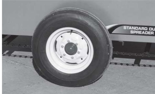
Wheel lug torque should be checked after every 50 hours of operation and tightened to the appropriate torque.
