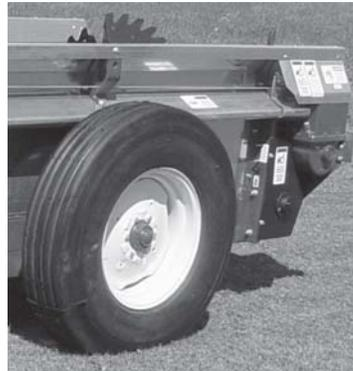
Wheel lug torque should be checked after every 50 hours of operation and tightened to the appropriate torque.
