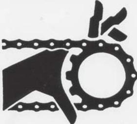
DO NOT CLEAN OR WORK ON THIS MACHINE WITHOUT FIRST DISENGAGING POWER AND SHUTTING OFF TRACTOR ENGINE.
