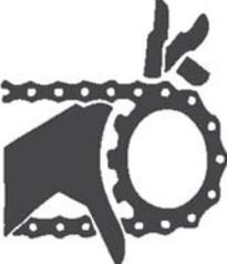
DO NOT OPERATE THIS EQUIPMENT IF THIS DECAL IS EXPOSED. REPLACE SAFETY SHIELDS.
