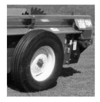
Wheel lug torque should be checked after every 50 hours of operation and tightened to the appropriate torque.
