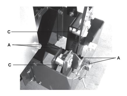
2 zerks located under shield on the pivot arm
