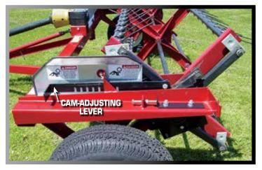
The angle of the rubber mounted teeth can be changed easily just by moving the handy lever to adjust the cam. Tedding will allow air to move through your hay for much faster drying, assuring uniform curing and higher quality hay.
