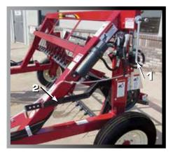
The **hand crank** (1) is for tedder reel height adjustment. The cam lever (2) is used to adjust the aggressiveness of the tedder teeth for a fluffier windrow.
