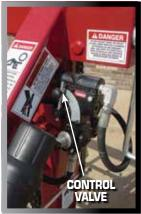
The speed of the tedder reel is hydraulically controlled.
