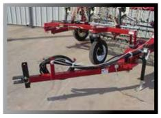
The **easy tongue adjustment system** is used to give the operator different offset positions for tedding and a position for storage.
