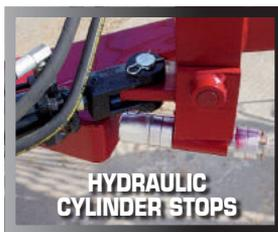
The **hydraulic cylinder** stops can be adjusted to limit the distance that the rake wheel arm swings out.
