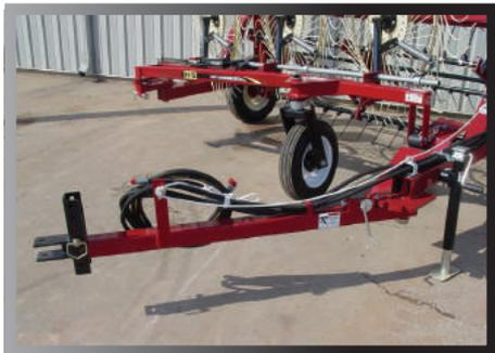
The **easy tongue adjustment system** is used to give the operator different offset positions for tedding and a position for storage.
