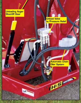
A slide style door provides easy opening for unloading. The automatic chain oiler system oils the drive chains when the discharged auger is raised.
