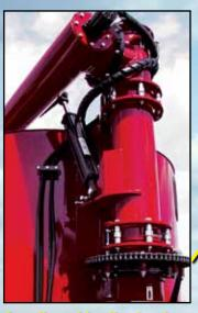
An adjustable alip eluten on the auger rotation provides protection if foreign objects are encountered.
