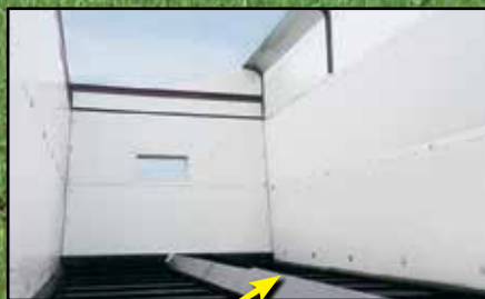
All Wide Body Boxes have Poly Bond plywood floors.
