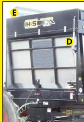
The **BIG DOG & TOP DOG** feature an electric actuator (D) and roof hood (E) as options.
