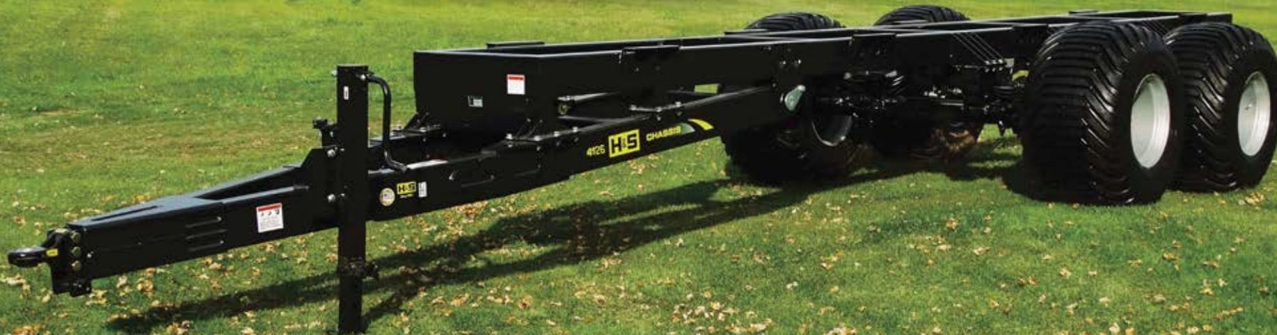
**13 ton per axle rating | 26-ton Spring Suspension System**
