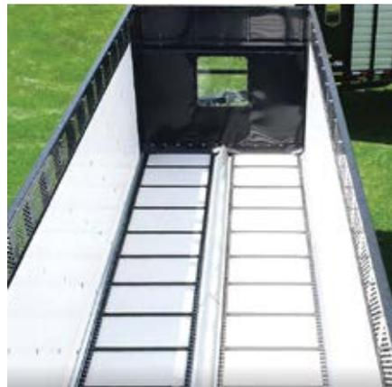
All **Wide Body** boxes have 1/2" thick virgin grade solid poly with rectangular tubular steel on the outside and C-channels in the center that run lengthwise under the floor for added strength.
