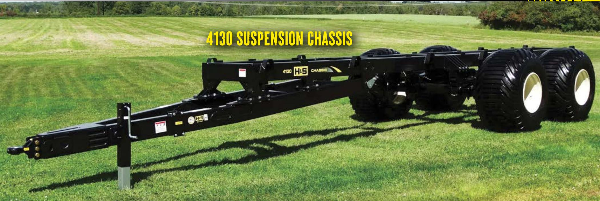
**15 ton per axle rating | 32-ton Spring Suspension System**
