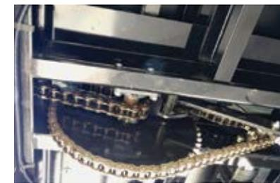
Spring-loaded tighteners are on the main apron drive for less stress on the main aprons upon engagement.
