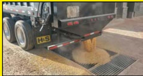
An optional quick-remove gravity unload grain hopper is available on **BIG DOG & TOP DOG** forage boxes that have a top pivot door.
