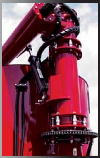
An adjustable slip clutch on the auger rotation provides protection if foreign objects are encountered.
